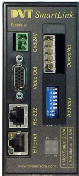
Figure 64: SmartLink with DeviceNet Connectivity
